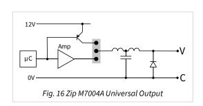
Connect the universal output to 0-10V DC motorised valve, 0-
