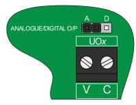
Universal Outputs are used as an analogue output in the range 0-10V, or as a switched 12VDC supply.
