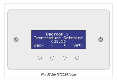
In automatic mode, the display allows the user to navigate up and down within the list of Essential Value pages and objects. It also allows the user to adjust the object values.
