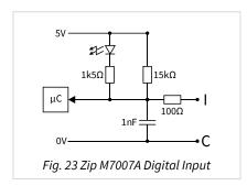
Each input has a two-way connector labelled **C** (common) and **I** (input). Each input also has a red LED, which lights when the contact closes. Each input senses the state of the contact and counts state changes (open-to-closed). Change rates up to 25Hz can be sensed (changes faster than this are taken to be noise).
