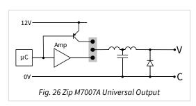
Connect the universal output to 0-10V DC motorised valve, 0-10V input on a variable frequency drive, 12V DC coil on an external relay, 12V DC indication lamp, etc.
