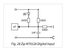
Each input has a two-way connector labelled **C** (common) and **I** (input). Each input also has a red LED, which lights when the contact closes. Each input senses the state of the contact and counts state changes (open-to-closed). Change rates up to 25Hz can be sensed (changes faster than this are taken to be noise).
