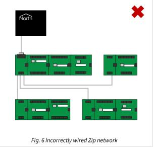
Recommended cables for wiring the Zip network are Belden 8761, Alpha Wire 2401C, or similar shielded twisted-pair cable (minimum 22AWG).
