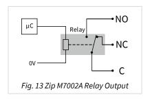
Each relay is rated 240V AC/28V DC at 10A resistive load. If higher loads are required, the relay can switch an external contactor.
