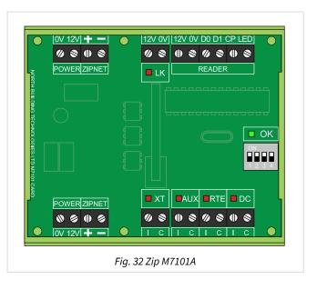
The module can monitor the security of its enclosure using either the on-board switch or external tamper input.
