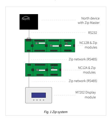
The Zip network is the link between the modules and the controller, called Zip Master. Any North device, such as Commander or ObSys, can be the Zip Master for a network.
