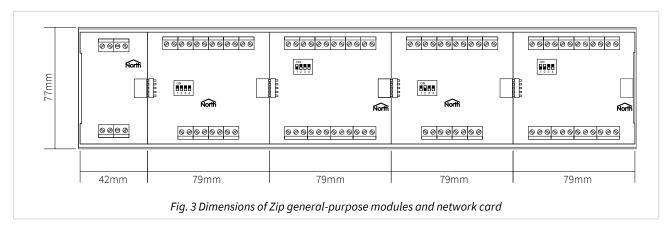
The total width for a network card and a maximum of four Zip modules will be:  $42mm + (4 \times 79mm) + (2 \times 2mm) = 362mm$
