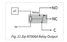
Connect the relay, for example, in-line with the power supply to an appropriate load such as a fan motor, motorised valve, lighting circuit, etc.
